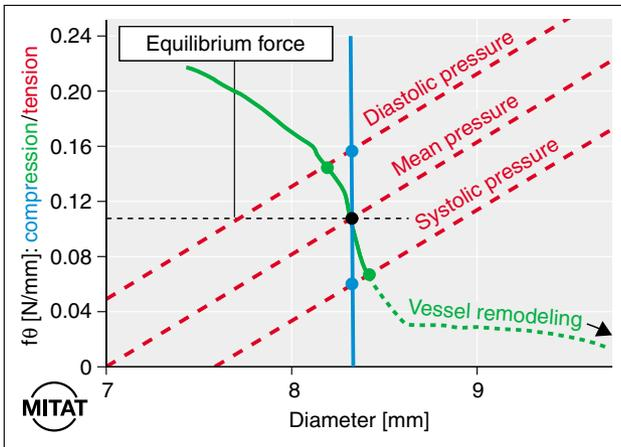
**Figure 8.** Dynamic effects on the vessel–stent interaction are exemplified by considering the effect of variations in the native vessel diameter on the equilibrium forces and equilibrium-stented vessel diameter. The red curves represent three native vessel diameters (diastolic, mid-cycle and systolic, for example). The blue circles illustrate the stented vessel equilibrium forces and diameters corresponding to a BE stent. The green circles correspond to an SE stent.
