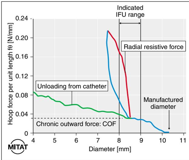
**Figure 5.** Hoop forces are measured during the release of a commercially-available, laser-cut Nitinol SE stent with a nominal 10 mm diameter. The release is halted at the centre of the intended diameter range of 8–9 mm, at which point the stent is compressed 1 mm in order to demonstrate biased stiffness. After the compression, the stent is again unloaded, quickly returning to the original unloading path, but with a small hysteresis.
