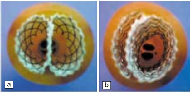
**Figure 3.** Two ‘kissing’ Nitinol stent grafts of equivalent radial stiffness, both shapes set to the same circular cross-section, but with different pinching stiffness. The design on the left can be crushed in any direction and will return to the desired shape shown. The design on the right prefers to buckle out of plane and return to a half-moon geometry, occluding one of the branches.
