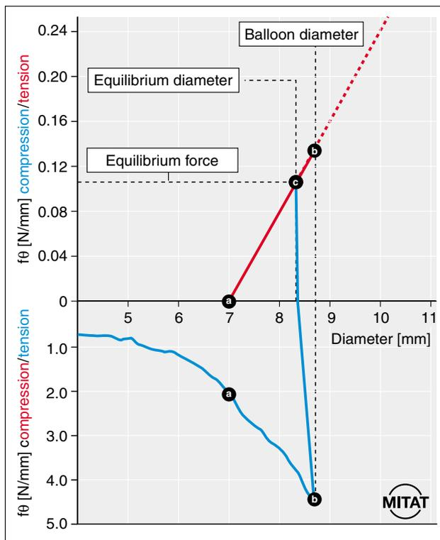
**Figure 7.** The same vessel as shown in Figure 6 is now stented with a typical SS laser-cut stent rated for use up to 9 mm and mounted on a non-compliant balloon. Inflation pressures far in excess of those shown in Figure 6 are required to bring balloon and stent to 9 mm (**c**). Deflation unloads the stent, then loads it in compression to the final equilibrium (**b**). (Note that the scale below the axis is much coarser than above.)
