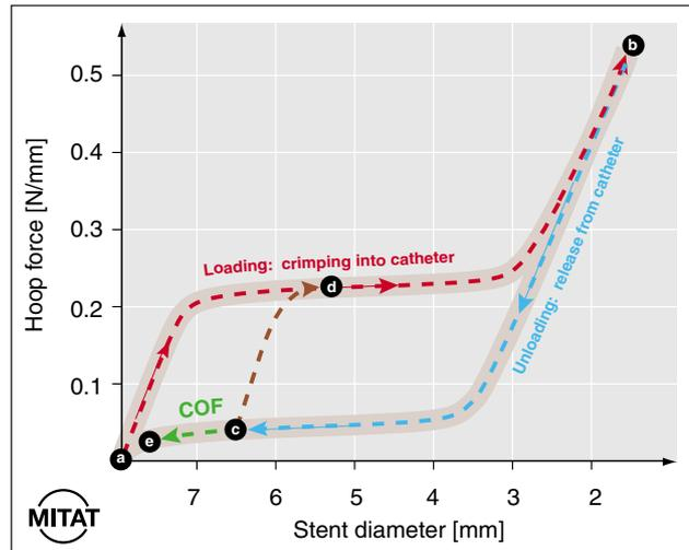
**Figure 4.** A typical superelastic stress–strain curve is transposed onto a hoop force–diameter diagram, illustrating the concept of ‘biased stiffness’. An 8 mm stent is compressed into a catheter (b), then released to a diameter (c). Further deformation forces are resisted by the ‘radial resistive force’ (d), while the opening ‘chronic outward force’ (COF) remains constant and gentle (e).
