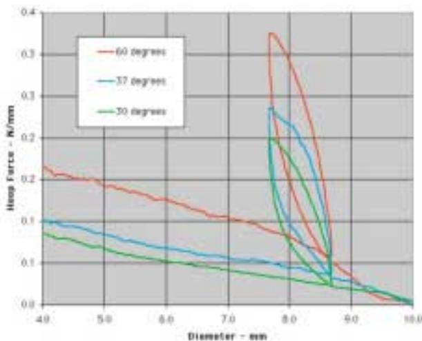
**Figure 12.** A commercially available 10 mm stent is unloaded in the same cycle as shown in Figure 5, but at three different temperatures. Note that the COF forces are increased by nearly 50% as the stent is warmed from  $30^\circ\text{C}$  to  $37^\circ\text{C}$ .
