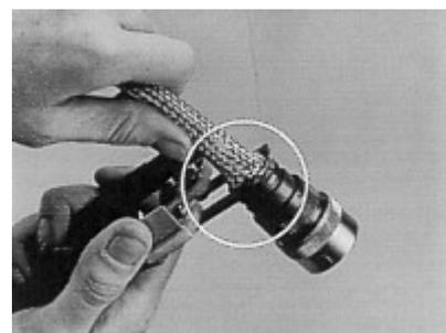
Fig. 13: Installing braid termination rings with conductive heating [12]
