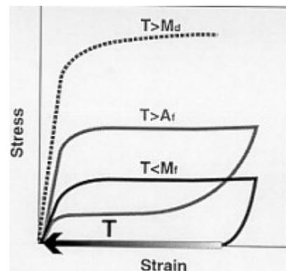
Fig. 2 (left): Schematic representation of the hysteresis loop
