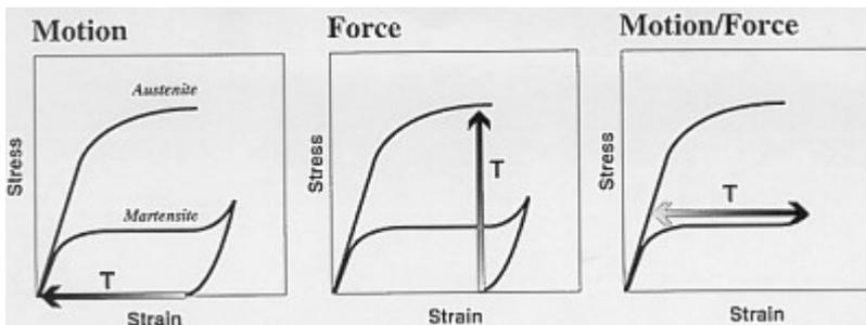
Fig. 6: Shape memory events in the stress/strain perspective [6]
