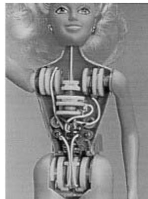
Fig. 27: Motion mechanism in toys
