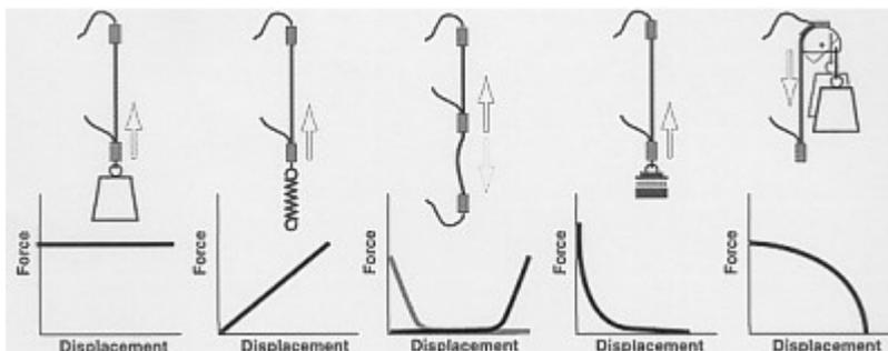
Fig. 7: Biasing Mechanisms and their effect on force/displacement characteristics [9]
