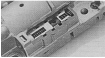
Fig. 18: Thermostatic control valve (cut-away)
