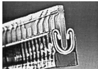
Fig. 17: Printed circuitboard connector [17]
