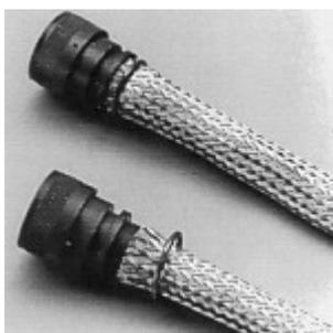
Fig. 12: Electromagnetic shielding braid termination with fastener rings [12]
