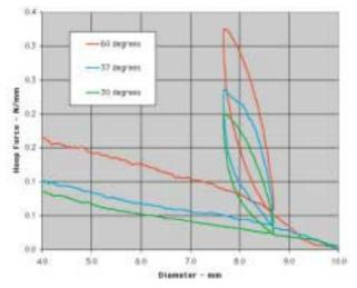
**Figure 12.** A commercially available 10 mm stent is unloaded in the same cycle as shown in Figure 5, but at three different temperatures. Note that the COF forces are increased by nearly 50% as the stent is warmed from 30° to 37°C.
