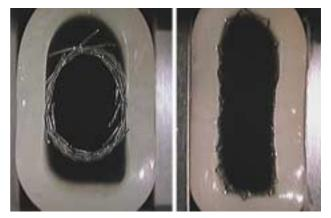
**Figure 11.** Two commercially available SE stents of the same nominal diameter are deployed into a flattened lumen. The stent on the right exhibits excellent wall apposition, while the one on the left does not.
