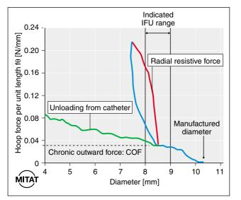
**Figure 5.** Hoop forces are measured during the release of a commercially-available, laser-cut Nitinol SE stent with a nominal 10 mm diameter. The release is halted at the centre of the intended diameter range of 8–9 mm, at which point the stent is compressed 1 mm in order to demonstrate biased stiffness. After the compression, the stent is again unloaded, quickly returning to the original unloading path, but with a small hysteresis.
