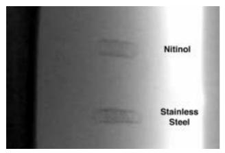
Figure 13. Two geometrically identical stents are viewed radiographically.
