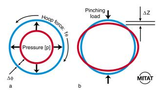
Figure 1. The two most common loading modes for stents are (a) radial or hoop and (b) pinching.
