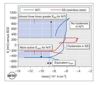
**Figure 2.** Representative cyclic polarisation curves for NiTi and SS in de-aerated Hanks solution at 37°C. Note the equivalent corrosion rate and the larger passive or corrosion resistant region exhibited by NiTi.
