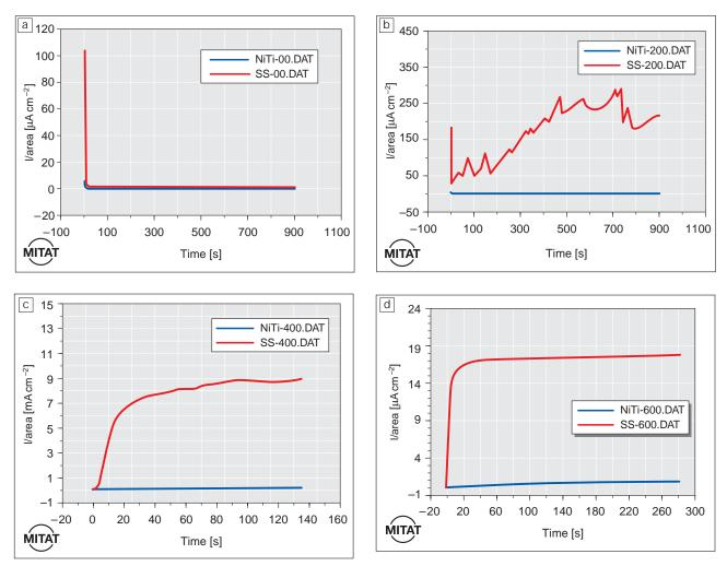
**Figure 3.** Representative scratch-testing data curves for NiTi and SS in de-aerated Hanks solution at 37°C. Current-density profiles are presented for (a) 0 mV potentiostatic hold, (b) 200 mV potentiostatic hold, (c) 400 mV potentiostatic hold, and (d) 600 mV potentiostatic hold.
