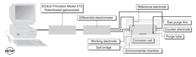
Figure 1. Generic schematic of experimental configuration used for corrosion testing.
