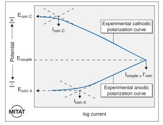
Figure 4. Schematic illustrating mixed-potential theory analysis.
