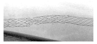
Figure 5. The popliteal is an example of a very dynamic artery, presenting a tremendous mechanical challenge for stent designers. Below is a fractured stent in the lower-central superficial femoral artery; the primary defomation mode in this case appears to be axial fatigue, caused by cyclic flexing in the knee. Such fractures appear to be common, but it is unclear what clinical impact they have, if any.
