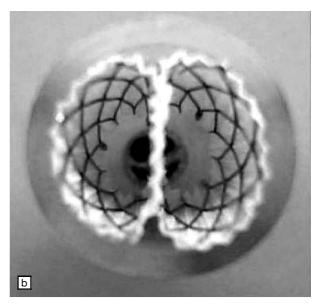
**Figure 3.** Buckling resistance, or strength, represents the true strength limitation of a BX stent, not radial strength. Even though SX stents cannot permanently buckle, (a) shows that certain superelastic stent designs can still buckle if pressured focally, in this case by a second, 'kissing' stent. Note that the design in (b), which as not buckled, actually has the greater radial stiffness — buckling resistance has little to do with radial stiffness or strength.
