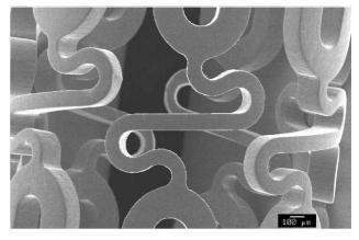
**Figure 4.** Very thin, easily deformed flexible links in the new generation of SS BX stents allows greatly improved flexibility and deliverability, rivaling that of SX stents.
